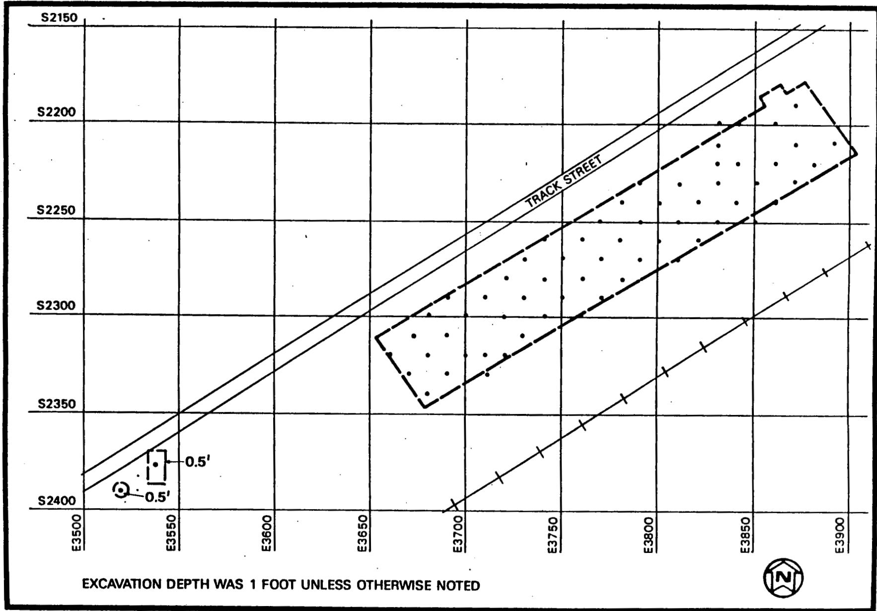
FIGURE 15 POST-REMEDIAL ACTION SAMPLING LOCATIONS ON PROPERTY N/N' SOUTH - SECTION 2
