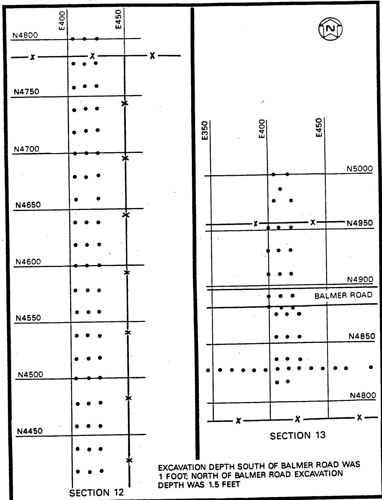
FIGURE 49 POST-REMEDIAL ACTION SAMPLING LOCATIONS ON THE CENTRAL DRAINAGE DITCH - SECTIONS 12 AND 13
